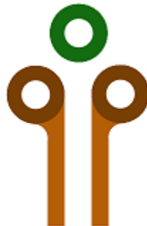
Figure 5.3: Single Ground Stitch Via
